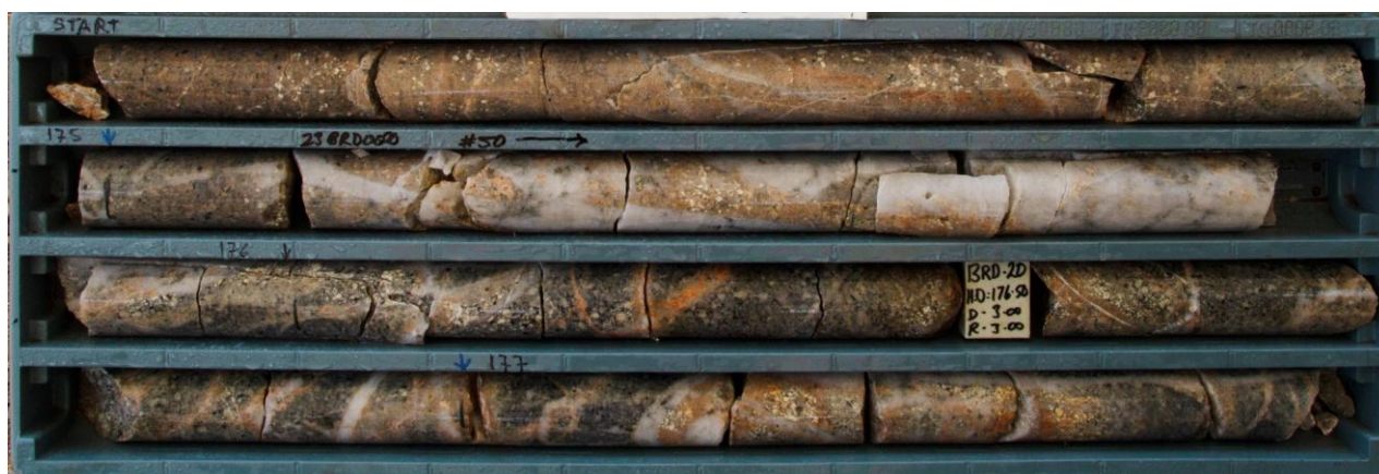
Figure 4 Strongly altered, quartz veined and mineralised porphyritic granodiorite in 23BRD0020 from 174.2m to 177.3m down-hole depth. Average assay for this interval is 0.59% Cu and 11ppm Mo.
