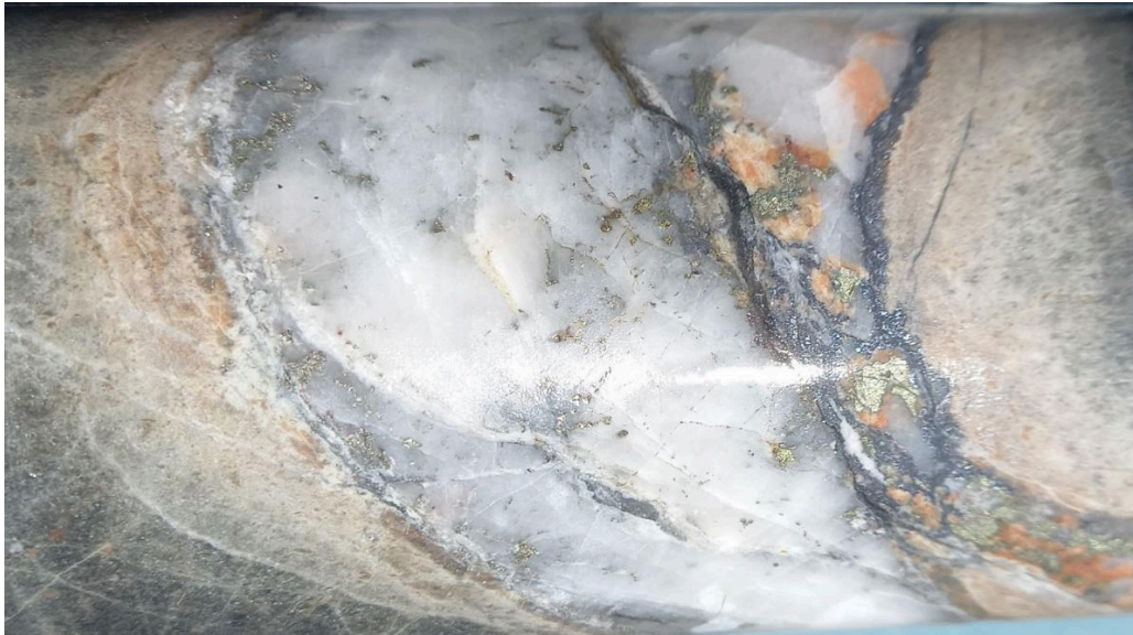
Figure 5 Quartz-molybdenite-chalcopyrite vein in potassic altered volcanic sediments, hole 23BRD0015 at 435m down-hole depth. Field of view approximately 15cm across.
