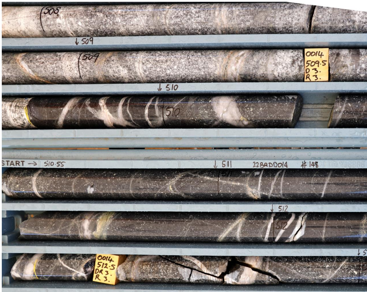
Figure 9 Dyke of porphyritic granite with potassic alteration intruding into volcanic sediments and fragmental rocks at 510m down-hole depth, 22BRD0014. Visually estimated chalcopyrite abundance ~0.3% by volume. HQ3 core (63.5mm diameter).*
