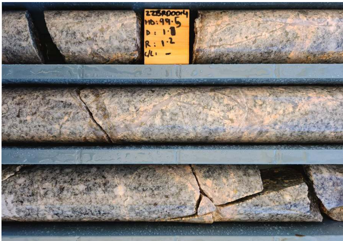
Figure 6 Porphyritic granodiorite cut by numerous quartz-chalcopyrite porphyry-style veins with orthoclase (potassic) alteration haloes. 22BRD0014 at approximately 100m down-hole depth. Visually estimated chalcopyrite abundance ~0.5% by volume. HQ3 core (63.5mm diameter).*
