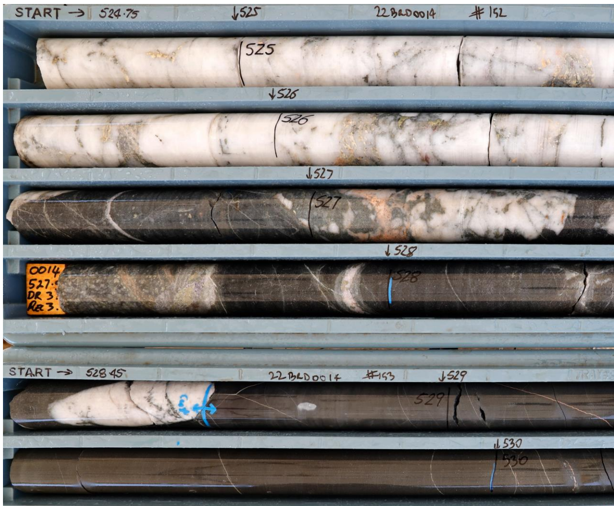
Figure 11 Thick quartz vein with minor coarse-grained chalcopyrite and zones of K-feldspar. Complex contact with volcanic sediments, truncated in turn by a post-mineral intrusion with contact at 528.6m down-hole depth. Visually estimated chalcopyrite abundance ~0.3% by volume. HQ3 core (63.5mm diameter).*
