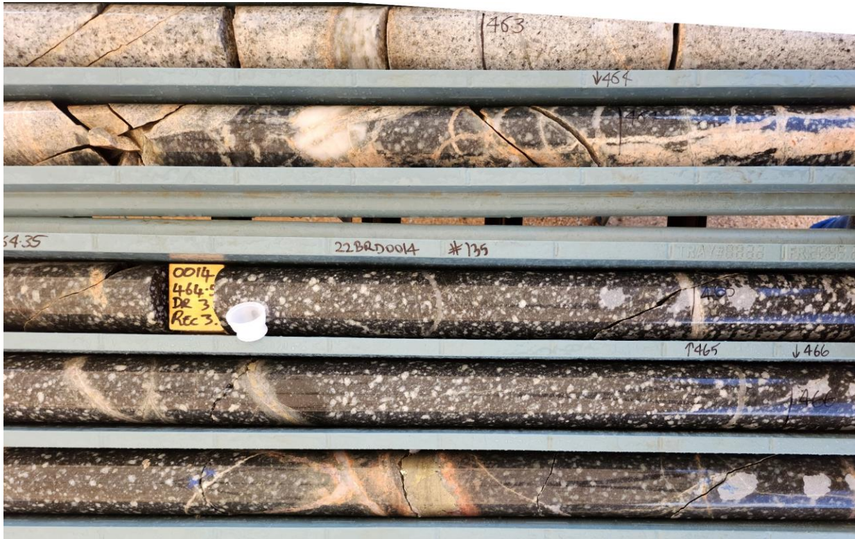
Figure 7 Multiple intrusions in 22BRD0014 at 465m down-hole depth. Upper part of photo shows porphyritic granite with quartz veins and potassic alteration. Lower part shows porphyritic granodiorite. All are cut by quartz veins with chalcopyrite and pyrite. Paler granite appears to intrude darker granodiorite, with chilled margins along contacts. Visually estimated chalcopyrite abundance ~0.5% by volume. HQ3 core (63.5mm diameter).*
