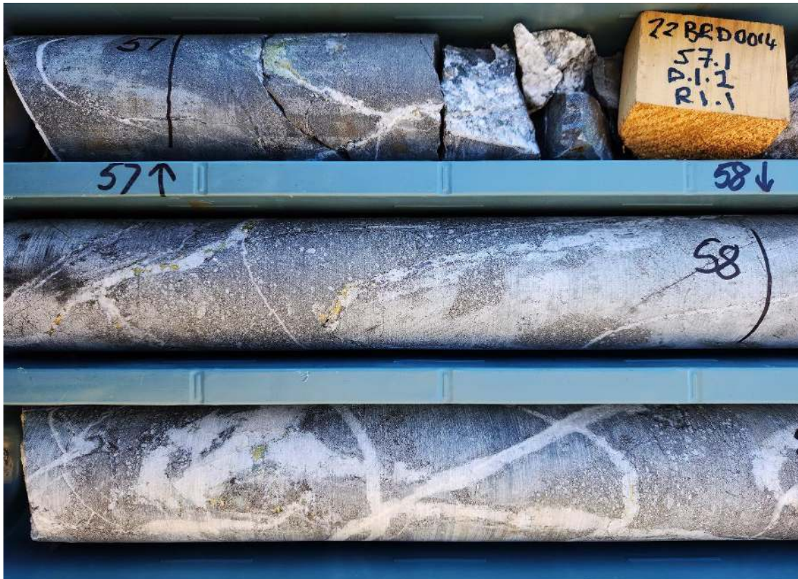
Figure 5 Quartz-chalcopyrite porphyry-style veins with minor chloritic alteration in porphyritic volcanoclastic host rocks. 22BRD0014 at 57-59m down-hole depth. Visually estimated chalcopyrite abundance ~0.3% by volume. HQ3 core (63.5mm diameter).*
