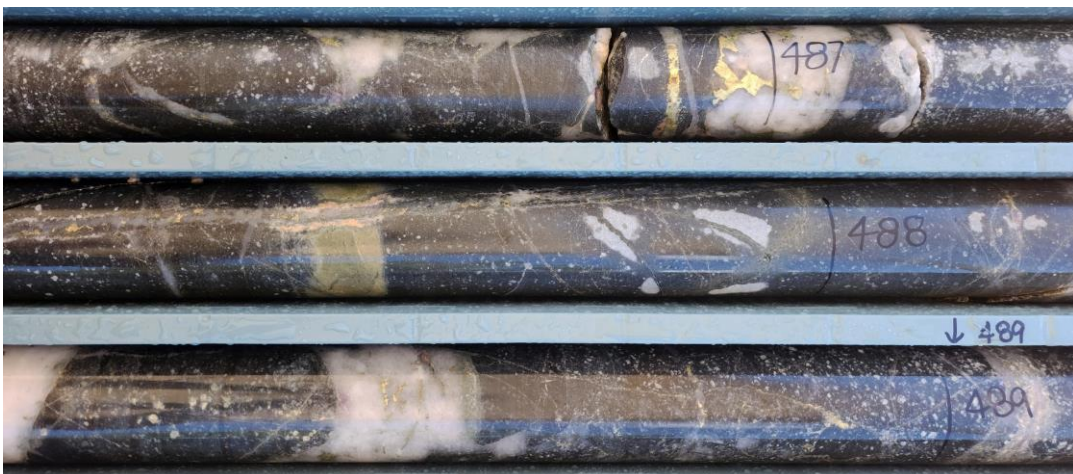
Figure 1 Mineralised drill core from 22BRD0014 between 486.5m and 489.0m down-hole depth. Note multiple phases of quartz-chalcopyrite \pm anhydrite \pm K-feldspar veining cutting weakly porphyritic volcanic-sediments/fragmental rocks. Visually estimated chalcopyrite abundance ~1% by volume. HQ3 core (63.5mm diameter).*
