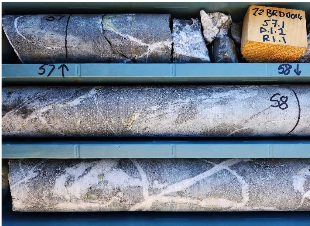
Figure 6 Quartz-chalcopyrite porphyry-style veins with minor chlorite after biotite alteration in porphyritic volcaniclastic host rocks. 22BRD0014 at 57-59m down-hole depth. HQ3 core (63.5mm diameter).
