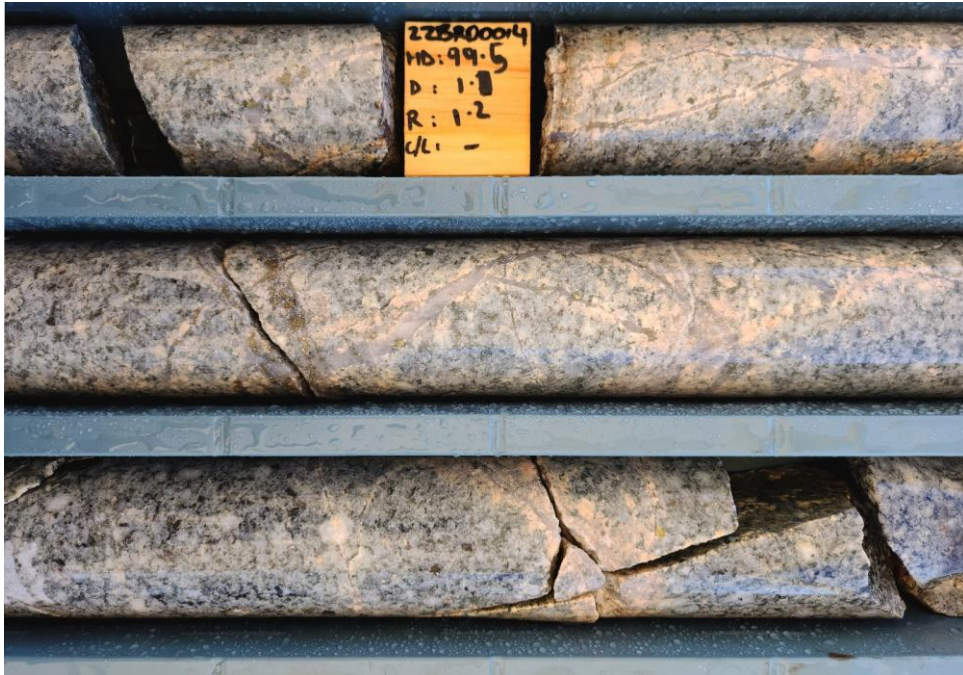
Figure 7 Porphyritic granodiorite cut by numerous quartz-chalcopyrite porphyry-style veins with orthoclase (potassic) alteration haloes. 22BRD0014 at approximately 100m down-hole depth. HQ3 core (63.5mm diameter).
