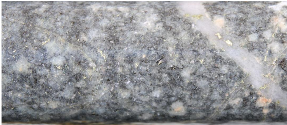
Figure 8 Porphyritic granodiorite cut by chalcopyrite in quartz veins and disseminated. 22BRD0014 at approximately 400m down-hole depth. HQ3 core (63.5mm diameter).
