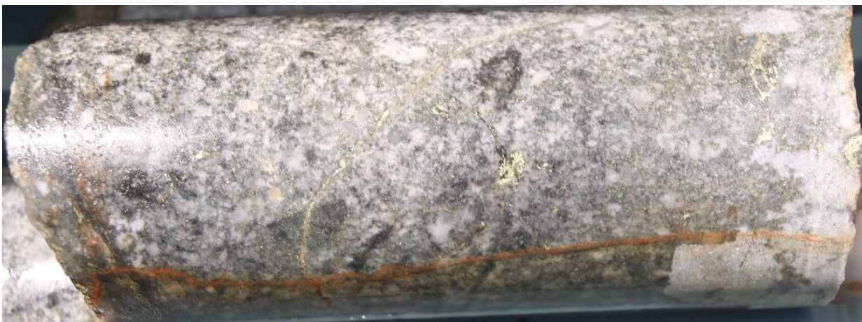
Figure 4 Coarse chalcopyrite veins and disseminations in porphyritic granodiorite. This photograph is from a 2m sample assaying 0.75% copper. Drill hole 22BRD0013 at ~434m down-hole depth. HQ3 core (63.5mm diameter).
