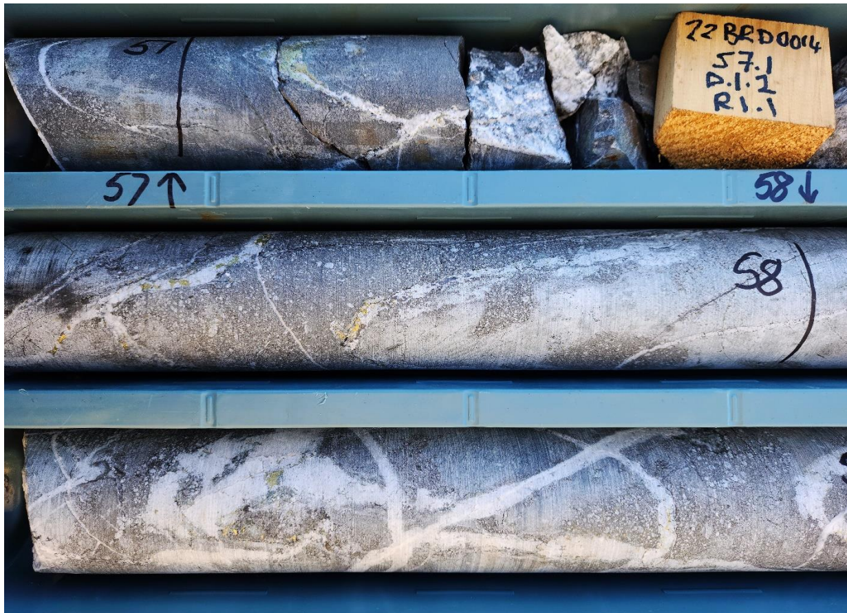
Figure 5 Quartz-chalcopyrite porphyry-style veins with minor chlorite after biotite alteration in porphyritic volcaniclastic host rocks. 22BRD0014 at 57-59m down-hole depth. HQ3 core (63.5mm diameter).
