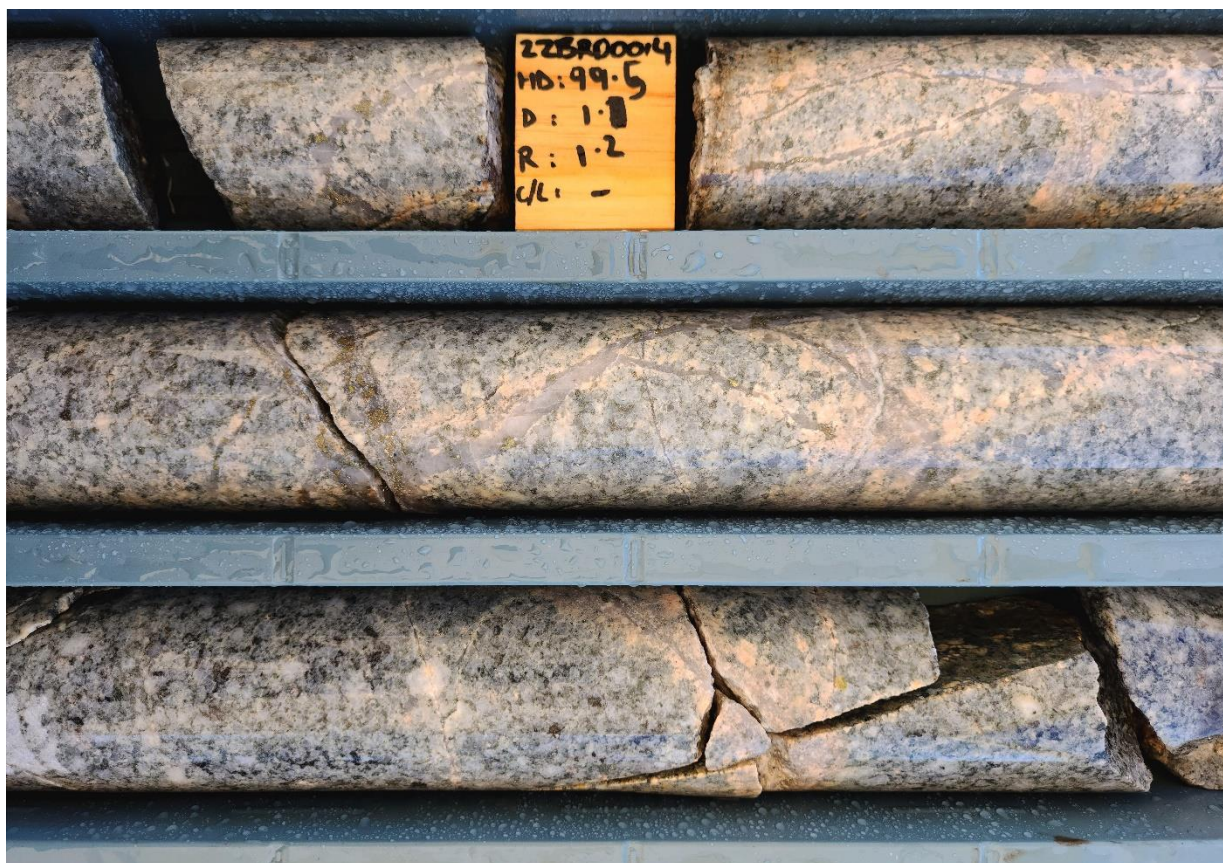
Figure 6 Porphyritic granodiorite cut by numerous quartz-chalcopyrite porphyry-style veins with orthoclase (potassic) alteration haloes. 22BRD0014 at approximately 100m down-hole depth. HQ3 core (63.5mm diameter).
