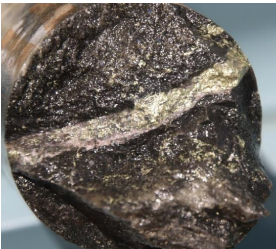
Figure 8 Coarse chalcopyrite and pyrite vein hosted in volcanic rocks in drill hole 22BRD0013 at 434.5m. HQ3 core (63.5mm diameter)
