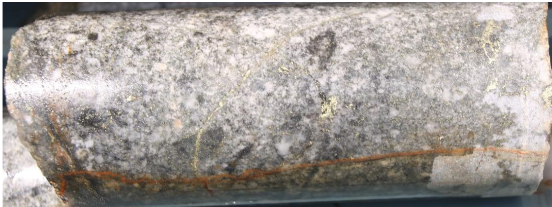
Figure 7 Coarse chalcopyrite veins and disseminations in porphyritic granodiorite in drill hole 22BRD0013 at ~434m. HQ3 core (63.5mm diameter)
