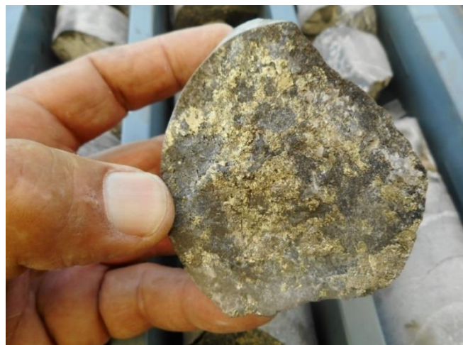
Figure 5 Coarse chalcopyrite associated with porphyry style quartz vein in drill hole 22BRD0013 at ~86m. HQ3 core (63.5mm diameter)
