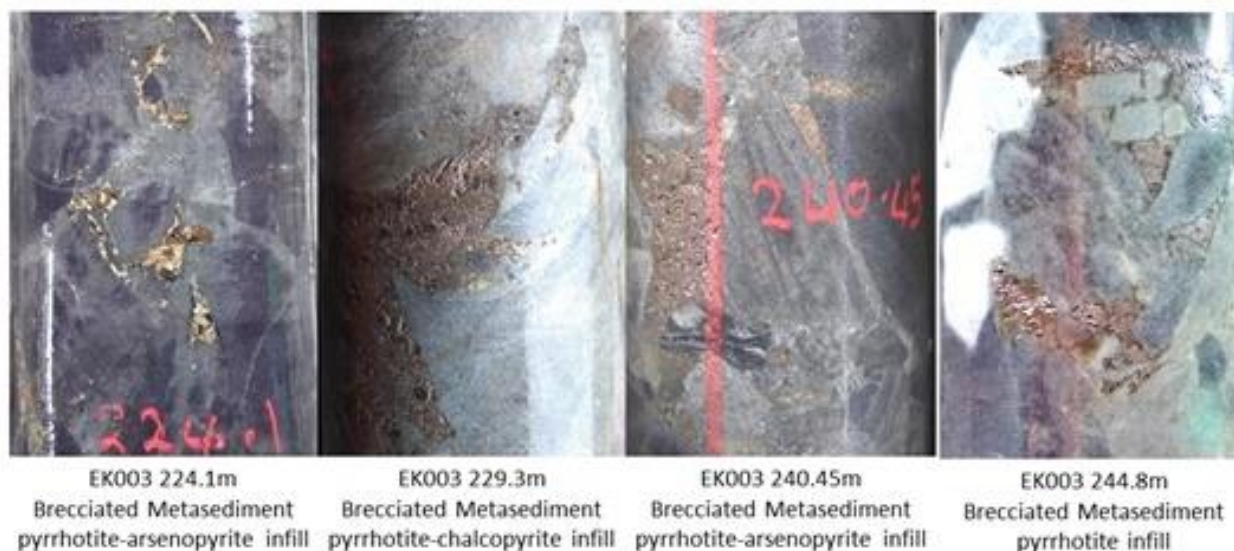
Figure 2 Selection of Core Photographs from EK003 Illustrating the Mineralised Interval of Brecciated Metasediment from 222.0m to 302.85m - May 2019
